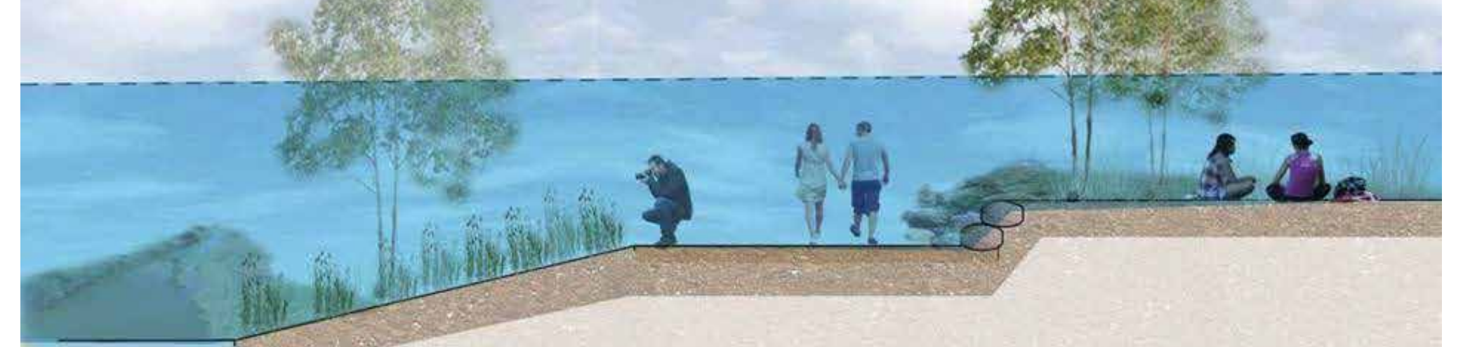
Conceptual section of the retention basin park "during the flood"
